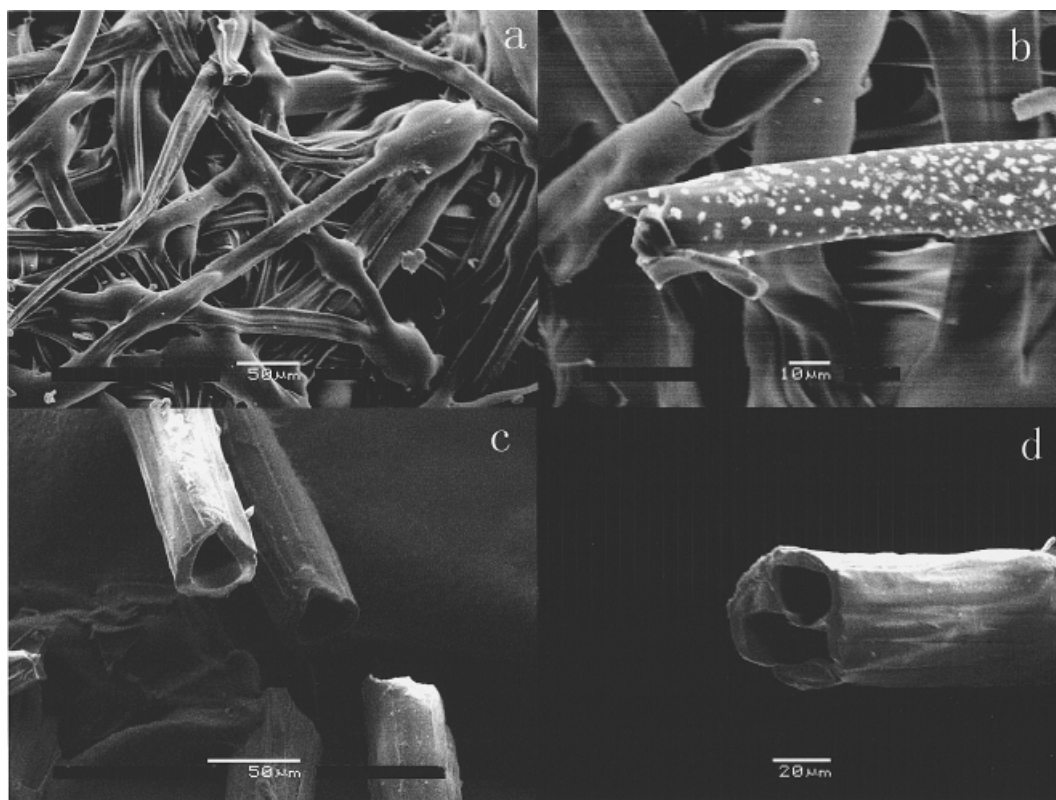
Figure 6 SEM images of surface of cocoon shell and section of raw silk fibers. (a,b) Shows B. mori cocoon shell treated at 350°C for 3 h; (c,d) shows B. mori raw silk fibers treated at 300°C for 3 h.
